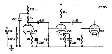
V<sub>1</sub> and V<sub>2</sub> are two units of 12AX7. V<sub>3</sub> is the succeeding stage.
